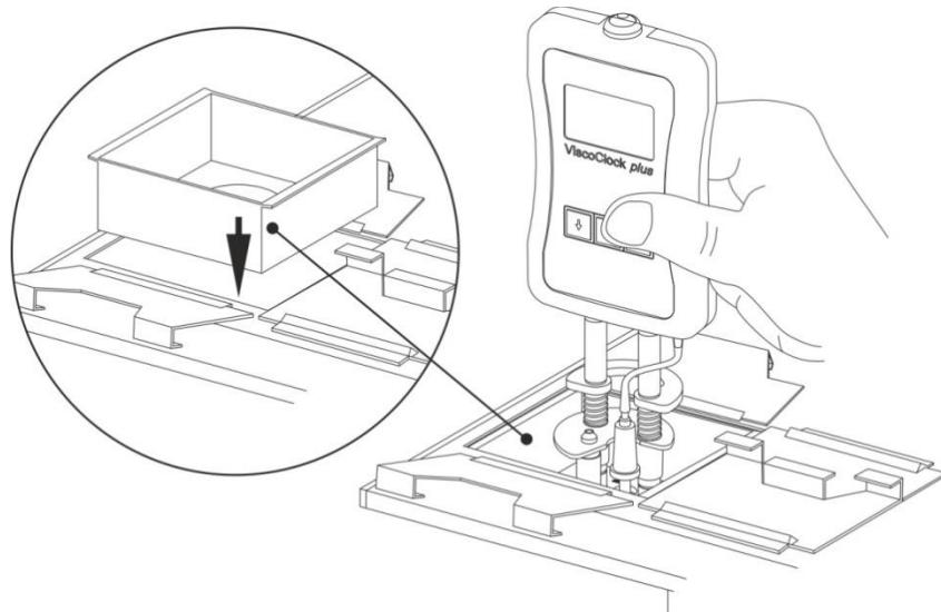
**Fig. 4 Placement of the ViscoClock *plus* into the thermostat bath**
