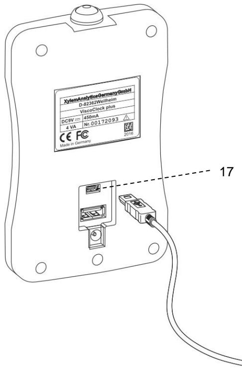
**Fig. 7 Connection of a peripheral via USB OTG cable VZ 6570 to the USB Mini-B connector (17) of the ViscoClock plus**
