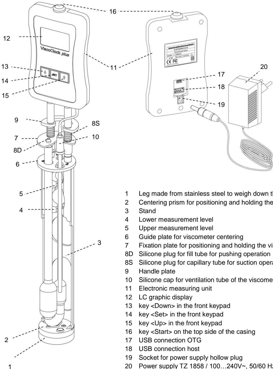
**Fig. 1 Description of the ViscoClock plus**
