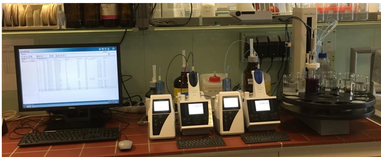
Figure 1: Complete set-up for an automated Kappa number determination
