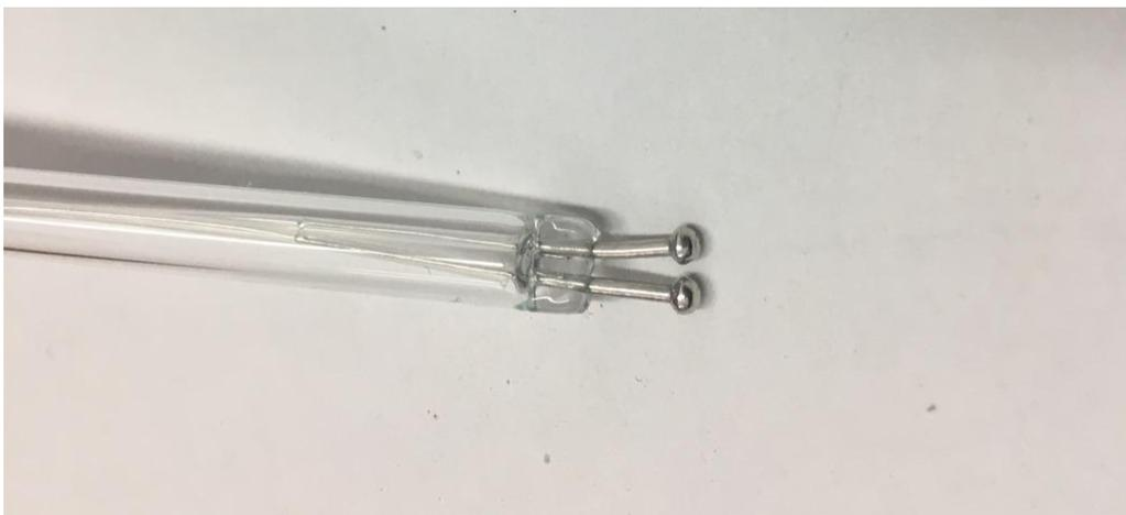
If the two platinum pins of the electrode are bent together, they can be carefully (!) bent apart.
