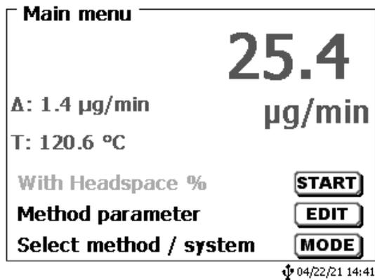
Various causes can be responsible for excessive drift - it is often used desiccant, a leaky titration cell, side reactions or even just a used reagent.
