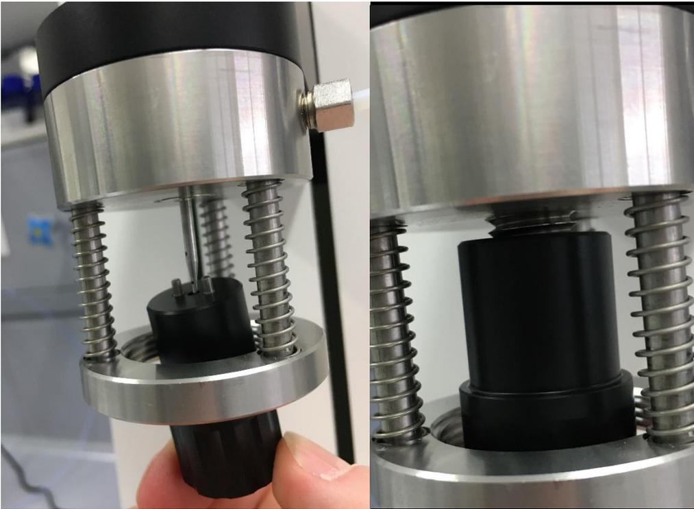
Now the needle can be removed, checked and cleaned if necessary. The inner needle (below) is only inserted through the outer needle.
