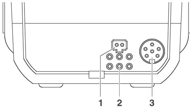
The diagram shows the rear panel of the device with three connection points labeled 1, 2, and 3. Point 1 is a power pack connector. Point 2 is a multi-pin contact point for LabStation operation. Point 3 is an RS232 serial interface connector.
