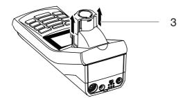
3 Open the external light cover (4) of the cell shaft.
