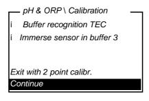
13 For two-point calibration, select with  $\langle A \rangle \langle \nabla \rangle$  *Exit with 2 point calibr.* and confirm with  $\langle START/ENTER \rangle$ .
