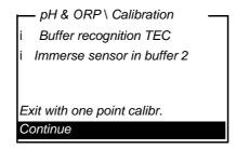
7 Single-point calibration: Using  $\langle \blacktriangle \rangle \langle \nabla \rangle$ , select *Exit with one point calibr.* and confirm with  $\langle$ **START/ENTER** $\rangle$ .
