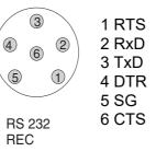
1 Connect the RS232 interface to the external printer with the AK540/ S cable.
