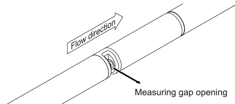
Fig. 3-1 Horizontal installation
