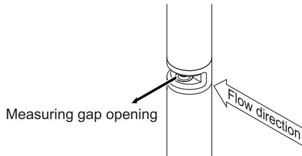
*Fig. 3-2 Vertical installation*
