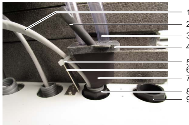
figure 3-25 Collection funnel for the common discharging of all liquids (lateral view)
