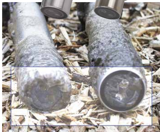
Sensor without and with ultrasound cleaning system after 30 days
