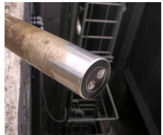
The optical windows of the VisoTurb® 700 IQ are clean even after several weeks of operation.
