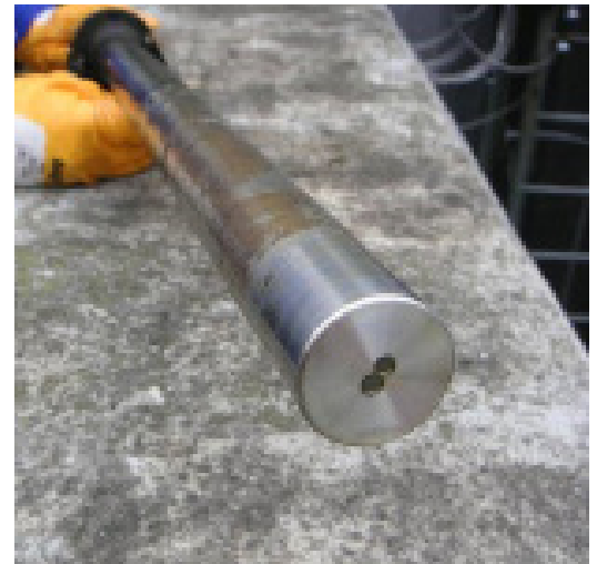
The optical windows of the ViSolid® 700 IQ are clean even after several weeks of operation.
