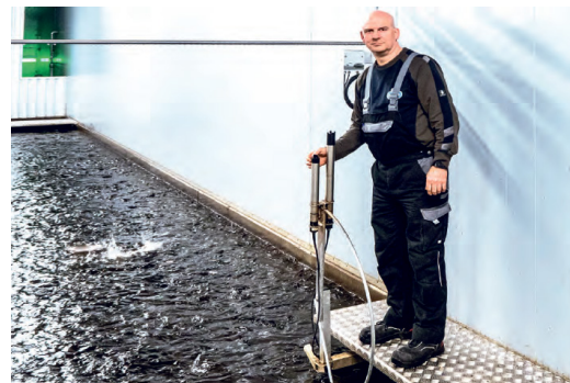
FREA fishing master Egon Folmer shows one of the special rotating brackets, on which a digital pH sensor SensoLyt® 700 IQ and the optical, calibration-free FDO® 700 IQ oxygen are mounted.
