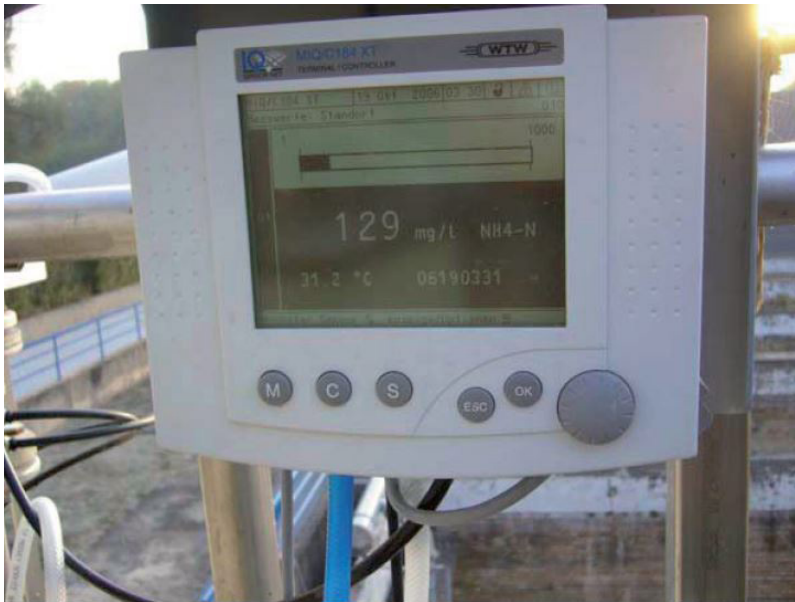
Fig. 4: NH 4 -N value measured with the VARiON® sensor
