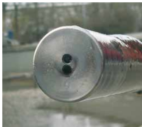
ViSolid® 700 IQ with working ultrasonic cleaning system shows no adverse effect.
