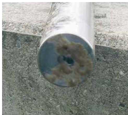
ViSolid® 700 IQ with switched-off cleaning system is completely covered with a biological layer after 16 days.
