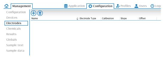
Use  $\oplus$  to add a new electrode. The name is freely assignable (here **Na 61**).
