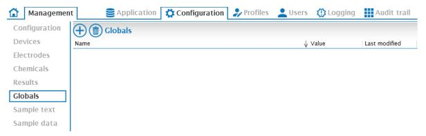
Press  $\oplus$  to add a new global. The name is freely assignable. The value of the global variable is editable but usually determined by an analysis (for example titration of a blank value).
