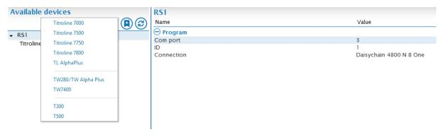
After selecting the desired device, it is listed under the RS port. The device address 0 is preset and must be adapted. In the following example a sample changer TW280 / TW alpha plus with address 3 was added.
