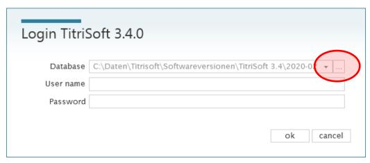
The selection of the database is only available here at the first start. Afterwards the database can be selected via the system settings in TitriSoft.
