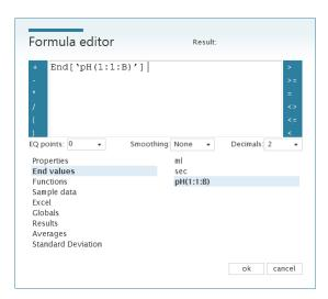
The numbers in brackets stand for: RS1, device address 1, measuring channel B.
