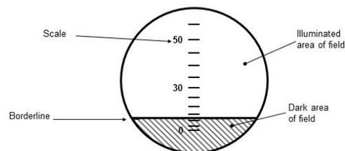
Bellingham + Stanley instruments also incorporate special software for interpreting 'fuzzy' borderlines that many products tend to produce. In this way, there is no subjective human judgement needed in taking a reading; a major advantage of an automatic instrument.
