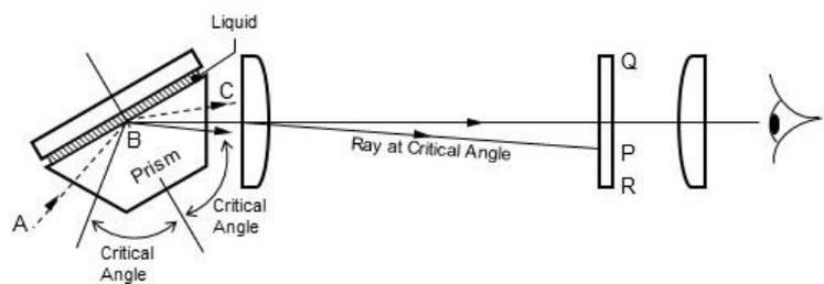
The RI of the sample is derived from the geometry of the optical path and the refractive index of the prism material.
