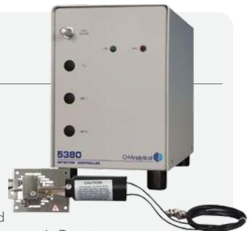
OI Analytical's patented 5380 Pulsed Flame Photometric Detector (PFPD) excels at selective, high sensitivity detection of sulphur, phosphorus, and other elements. The 5380 PFPD provides a 10–100x increase in signal-to-noise and a 10x increase in selectivity over traditional Flame Photometric Detectors and requires significantly less maintenance and gas to operate.
