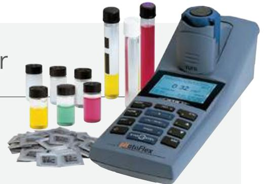
The portable colorimeter series of pHotoFlex offer more than 135 Standard parameters for water, food, beverage and aquaculture. With optional docking station and pH or Turbidity (IR) measurement, these "real" multi-parameter instruments cover up to three analyses in just one meter!
