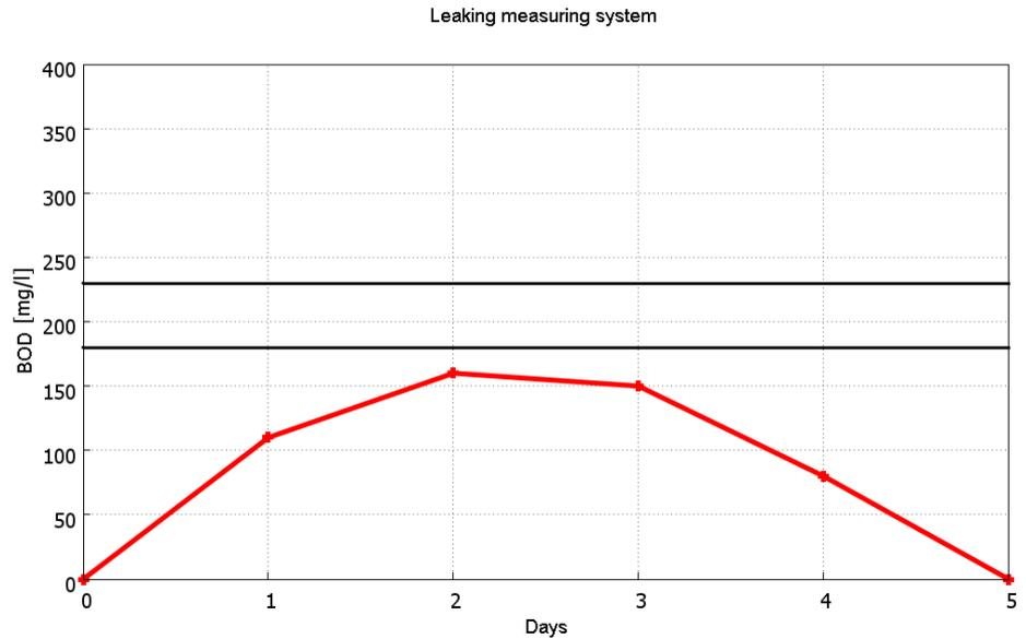
Leaking measuring system. Replace the rubber sleeve or the seal on the measuring head.
