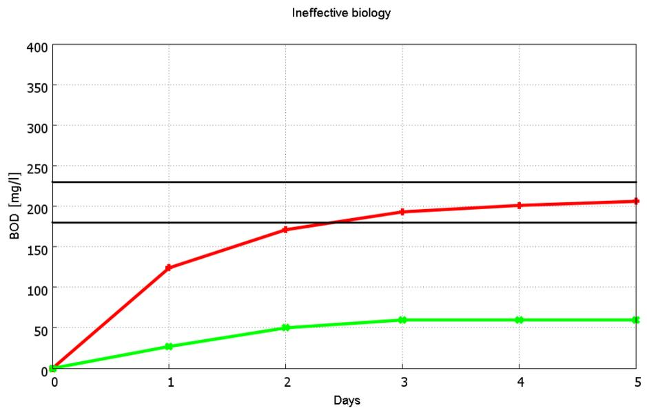
The upper curve shows the normal progression of a BOD measurement. In the lower curve the biology employed was not effective enough. It may have been inhibited by wastewater constituents. Carry out the BOD determination according to the application report [\[Inhibiting and toxic substances\]](#).
