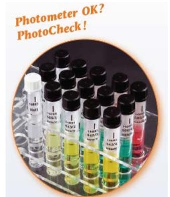
Especially for spectrophotometers, there are a lot of highly sophisticated tools, reaching from glass to liquid filters provided by different manufacturers for testing wavelength accuracy, stray light, reproduceability etc. Many meters, like WTW's photoLab® 7600 UV-VIS are supporting the AQA tools by specific and easy to handle menus.
