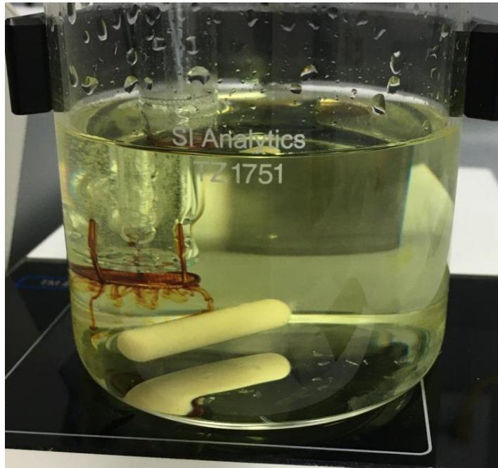
If only a few gas bubbles form and no brown clouds, the generator electrode or the electrode cable is defective and must be replaced.
