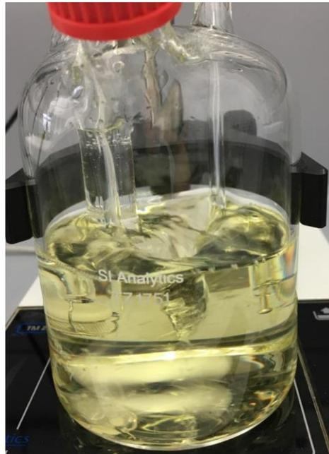
If there are problems with the coulometric KF titration, a water standard (a standard with a concentration of 1 mg / g is recommended) should be titrated first to exclude that only the sample matrix leads to problems.
