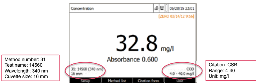
Fig. 10 photoLab® 7000 Series - Display: Beside the COD value, additional information are displayed
