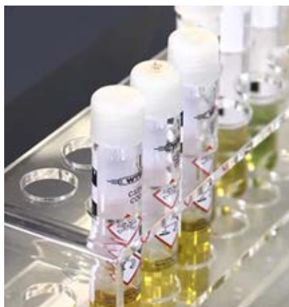
Fig. 2 COD test in three-fold determination
